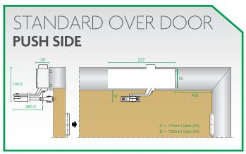
Provided the site conditions allow, an opening angle of 180 degrees is possible with this installation. Please note that using measurements A or B will provide different spring strengths.
