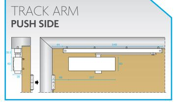
Provided the site conditions allow, an opening angle of 160 degrees is possible with this installation. Please note that using this installation a size 3 spring strength is achieved.
