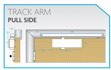
Provided the site conditions allow, an opening angle of 180 degrees is possible with this installation. Please note that using this installation a size 3 spring strength is achieved.
